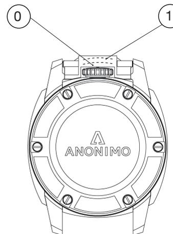
Position 0: The watch is working and water resistance is guaranteed. The crown is locked thanks to the patented protective lever.
